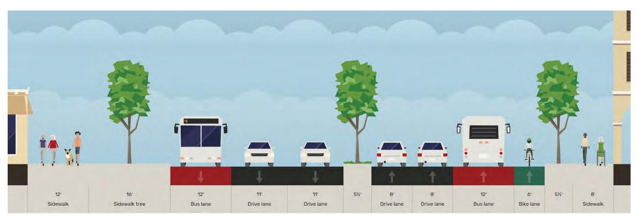
Figure 38. Proposed phase II treatments for segment A Made on Streetmix.net
