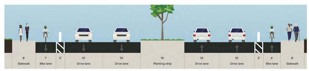
Figure 53. Segment C, Phase I street reconfiguration cross-section Made on Streetmix.net
