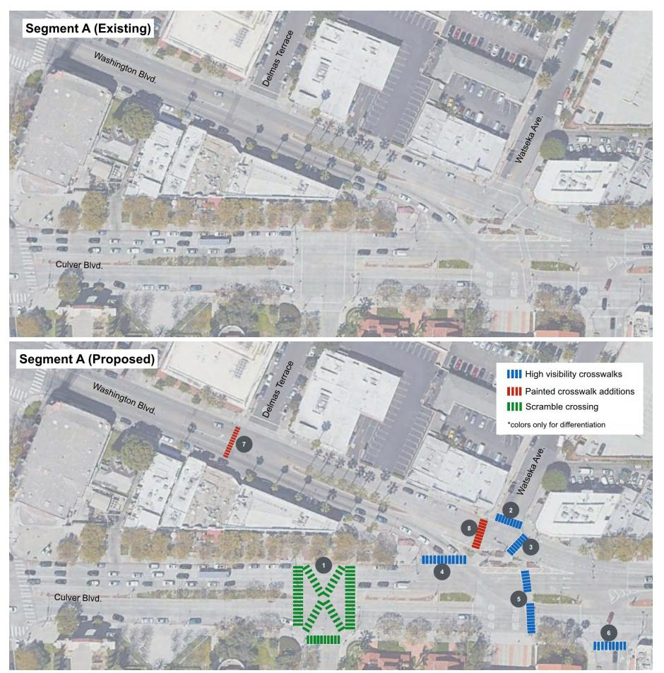
(Top) Figure 31. Existing conditions of segment A (Bottom) Figure 32. Proposed Phase I treatments for segment A
