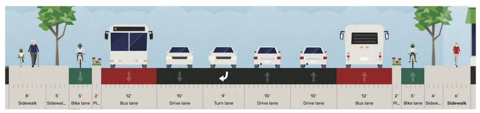
Figure 77. Segment B, Phase III street reconfiguration cross-section. Made on Streetmix.net.
