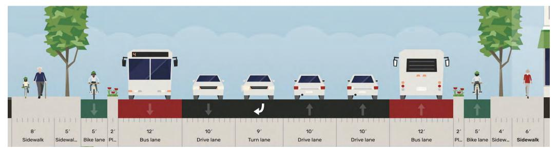
Figure 74. Segment A, Phase III street reconfiguration cross-section. Made on Streetmix.net.
