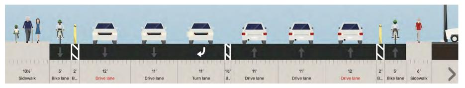
Figure 63. Segment B, Phase II street reconfiguration cross-section. Made on Streetmix.net
