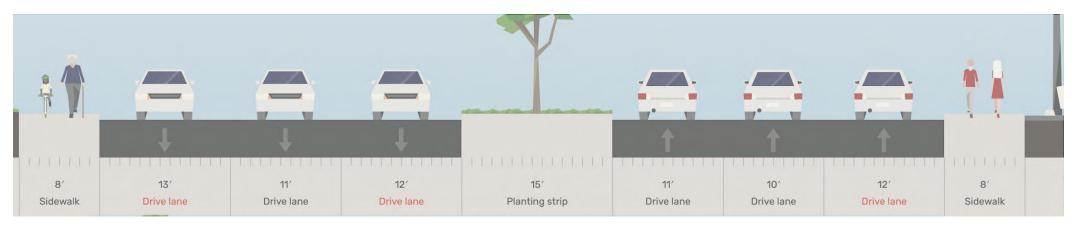
Figure 79. Segment C, existing street cross-section. Made on Streetmix.net.
