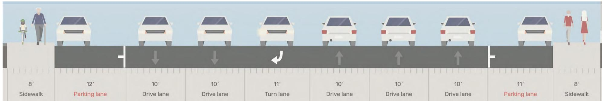
Figure 59. Segment A, existing cross-section Made on Streetmix.net
