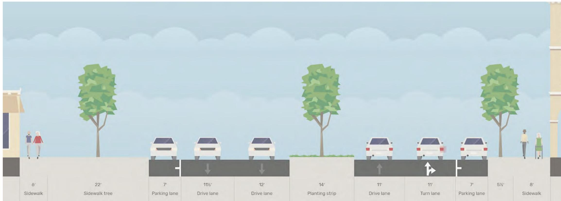
Figure 37. Existing condition Culver Blvd. & Lafayette Pl. (Segment A) Made on Streetmix.net
