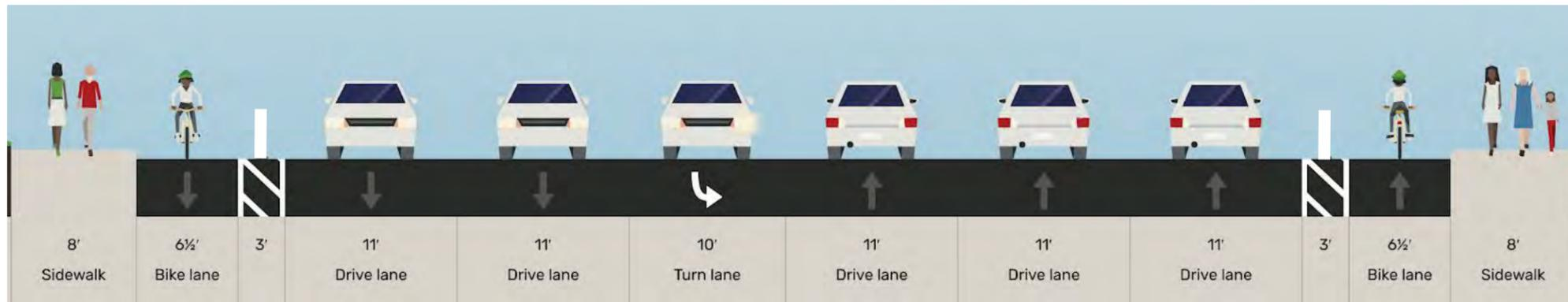
Figure 47. Segment A, Phase I street reconfiguration cross-section. Made on Streetmix.net
